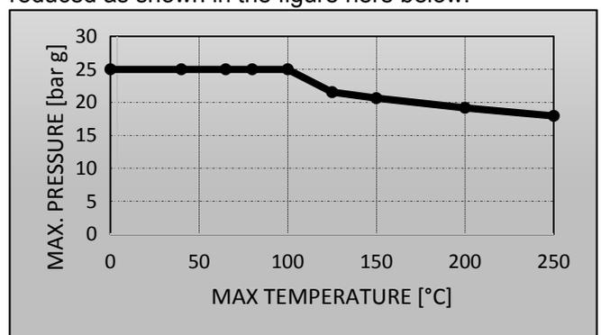
**However, if the filter is used at temperatures above 100 ° C contact Asco Filtri.**
