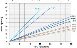
For liquid with different viscosity than water, multiply the Delta-P by the liquid viscosity in cP.
